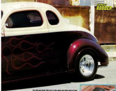
The '32 was lowered .500 inch to 320 inches and fitted with a Crown Cam and offset, forged V16 3.27 pistons, stainless Inconelone Mark Nutter headers, a Holley 650-cfm carb, and Edelbrock aluminum rock covers. Power goes to a Turbo 400 and a Detroit Locker Four disc clutch over 3.70 gears.
